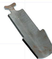
Piece of steel welded on to front of opener to protect liquid line from trash CZD0EF
